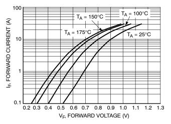
Figure 1. Typical Forward Voltage
