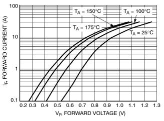
Figure 2. Maximum Forward Voltage
