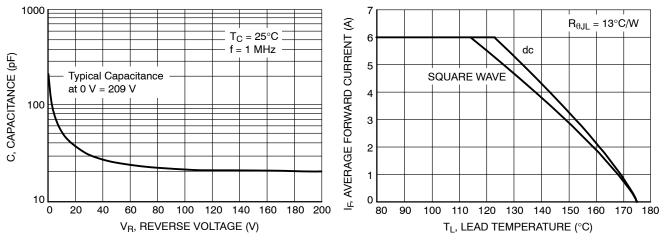
Figure 5. Typical Capacitance
