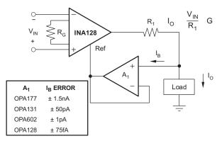
Figure 34. Differential Voltage to Current Converter
