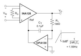
Figure 32. AC-Coupled Instrumentation Amplifier
