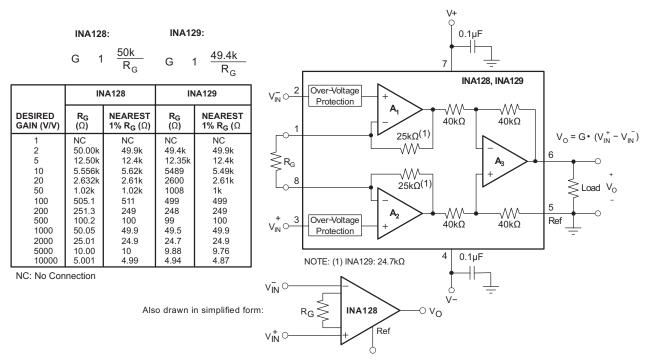
Figure 24. Basic Connections
