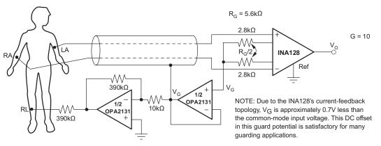
Figure 35. ECG Amplifier With Right-Leg Drive
