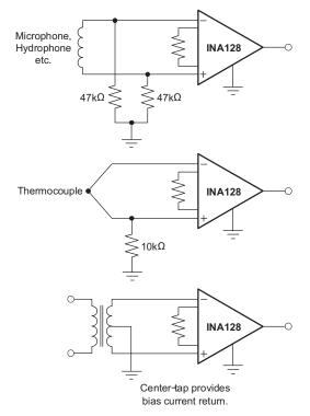
Figure 26. Providing an Input Common-Mode Current Path
