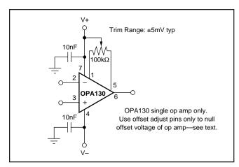
FIGURE 1. OPA130 Offset Voltage Trim Circuit.
