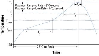
Note: All temperatures refer to the center of the package, measured on the capacitor body surface that is facing up during assembly reflow.
