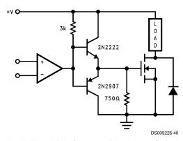
FIGURE 12. High Current, High Voltage Switch
