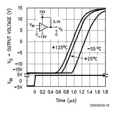
Comparator Response Times — Non-Inverting Input, Negative Transition
