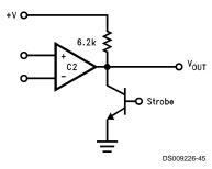
FIGURE 16. Basic Comparator with External Strobe
