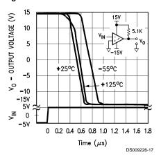
Comparator Response Times—Non-Inverting Input, Positive Transition
