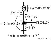
FIGURE 1. Voltage Associated with Reference (current source I, is external)
