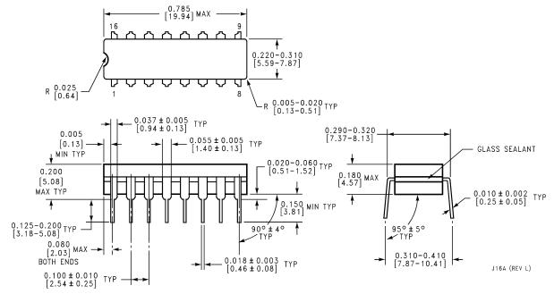
16-Lead Ceramic Dual-In-Line Package (J)
