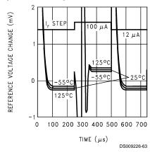
Reference Step Response for 100  $\mu$ A  $\sim$  10 mA Current Step
