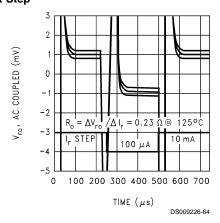
Reference Voltage Change with Supply Voltage Step
