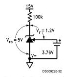
FIGURE 4. Thevenin Equivalent of Reference with 5V Output
