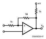
FIGURE 18. Comparator with Hysteresis ( $\triangle V_H = {}^+V(1k/1M)$ )
