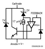
FIGURE 2. Reference Equivalent Circuit
