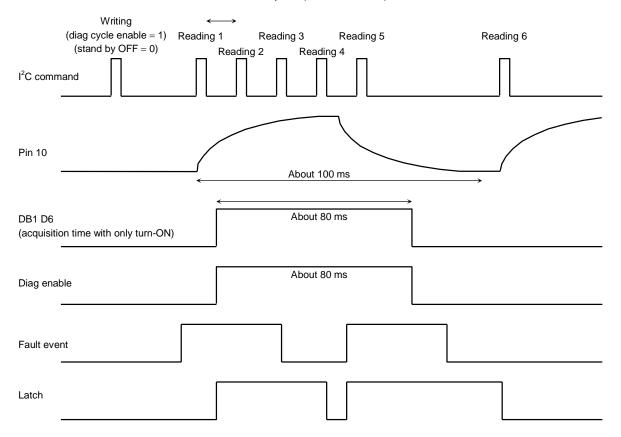
The turn ON diagnostic acquisition time is determined by the ripple filter capacitance C2 and the equivalent internal resistance Rr as below expression.
