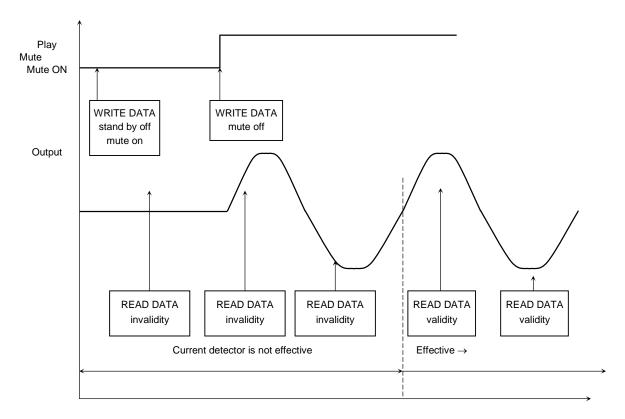
Figure 10 Tweeter Open Detection Timing Chart
