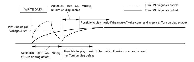
Figure 11 Automatic Turn on Muting Timing Chart
