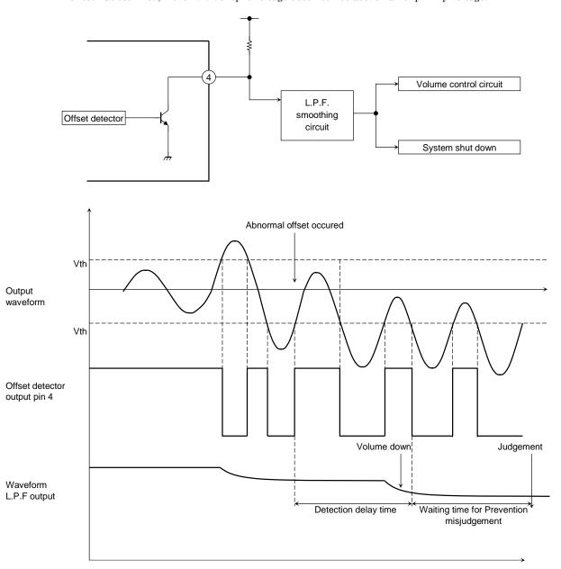
Figure 9 Hardware Output Offset Detection
