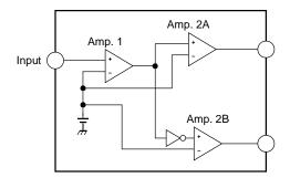
Figure 1 Block Diagram
