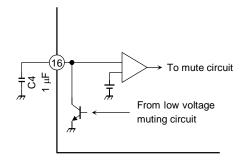
Figure 2 Pin 16 Muting Circuit
