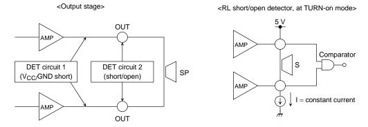
The comparator detect the voltage between speaker both ends.
