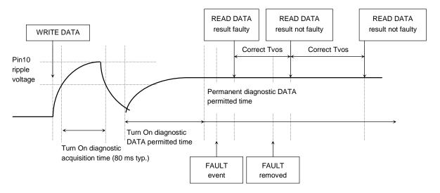
Figure 8 Software Output Offset Detection Timing Chart
