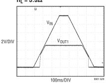
Channel 2 Start-Up and Dropout,  $R_L = 20\Omega$
