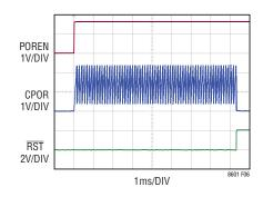
Figure 6. Power-On Reset Timing
