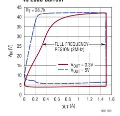
Channel 2 Full Frequency VIN vs Load Current
