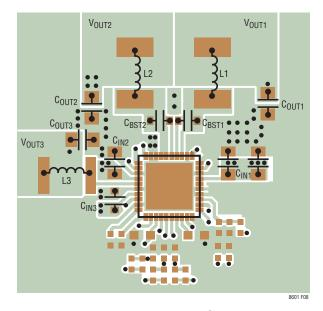
Figure 8. Recommended PCB Layout
