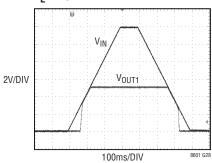
Channel 1 Start-Up and Dropout,  $R_L = 3.3\Omega$
