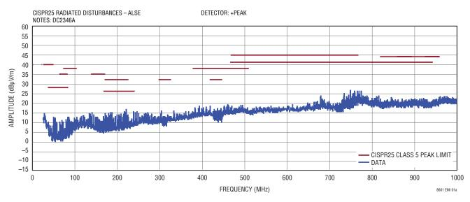
Demo Board with EMI Filter Installed,  $14V_{IN}$ , 1A on All Outputs,  $f_{SW} = 2MHz$ .
