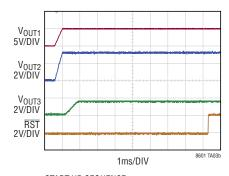
START-UP SEQUENCE: CH1 AND CH2 SOFT-START RATIOMETRICALLY; THEN CH3 TURNS ON; THEN POR TIMER STARTS.
