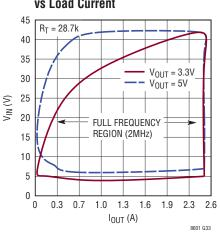
Channel 3 Full Frequency VIN vs Load Current
