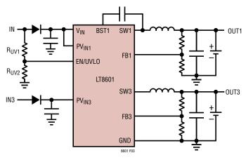
Figure 3. Reverse Protection Diodes
