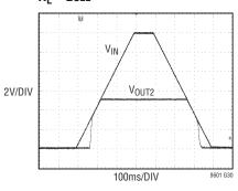
Channel 2 Start-Up and Dropout,  $R_L = 2\Omega$
