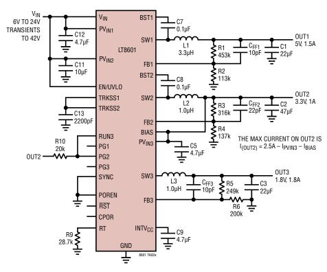
THE VALUES SHOWN ARE FOR 2MHz OPERATION. FOR 1MHz OPERATION, MAKE THE FOLLOWING CHANGES: L1 = 6.2 $\mu$ H, CFF1 = 4.7pF, L2 = 2.7 $\mu$ H, L3 = 2.2 $\mu$ H, R9 = 60.4k. AT 1MHz OPERATION, THE INPUT VOLTAGE RANGE IS 6V TO 42V.
