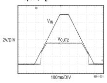
Channel 1 Full Frequency VIN vs Load Current
