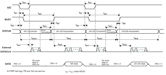
Figure 3. Basic Conversion Timing (External DATACLK)
