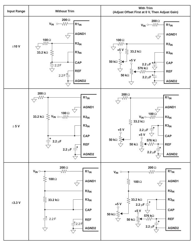
Figure 30. Offset/Gain Circuits for Bipolar Input Ranges
