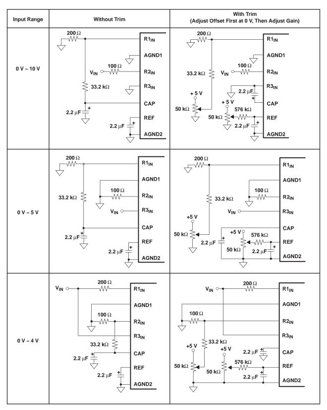
Figure 29. Offset/Gain Circuits for Unipolar Input Ranges
