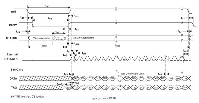
Figure 4. Read After Conversion (Discontinuous External DATACLK)
