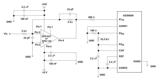
Figure 28. Typical Driving Circuitry (±10 V, No Trim)
