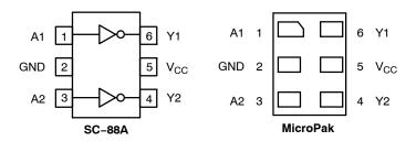
Figure 1. Pinout Diagrams (Top Views)
