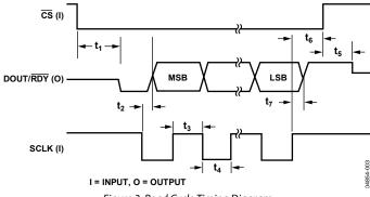
Figure 3. Read Cycle Timing Diagram
