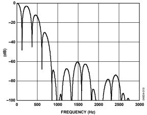
Figure 15. Filter Response with Update Rate = 242 Hz (Chop Enabled)
