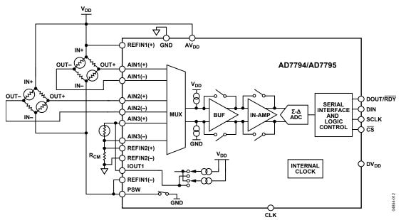
Figure 12. Basic Connection Diagram
