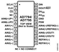
Figure 5. Pin Configuration
