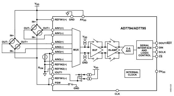
Figure 24. Typical Application (Flowmeter)
