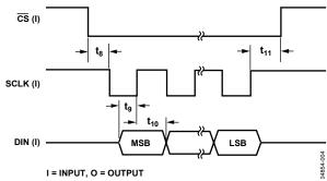
Figure 4. Write Cycle Timing Diagram
