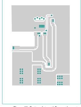
Figure 28. Bottom Internal Copper Layout
