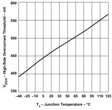
Figure 10. High-Side Overcurrent Threshold vs Junction Temperature
