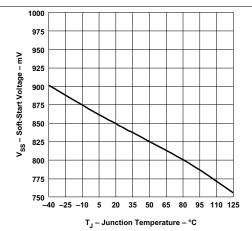
Figure 12. Soft-Start Voltage vs Junction Temperature
