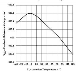
Figure 7. Feedback Reference Voltage vs Junction Temperature
