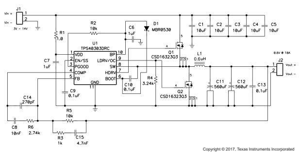
Figure 22. TPS40303 Design Example Schematic
