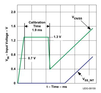
Figure 13. Start-Up Sequence and Timing
