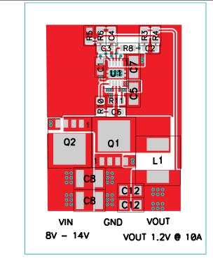
Figure 26. Top Copper With Components
