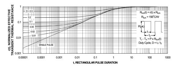
Figure 11. Transient Thermal Response Curve
