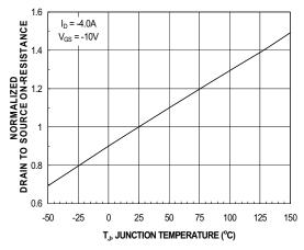
Figure 3. Normalized On-Resistance vs Junction Temperature
