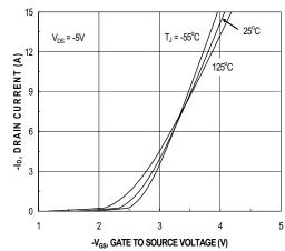
Figure 5. Transfer Characteristics
