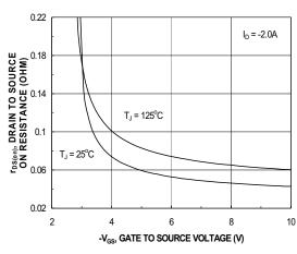
Figure 4. On-Resistance vs Gate to Source Voltage
