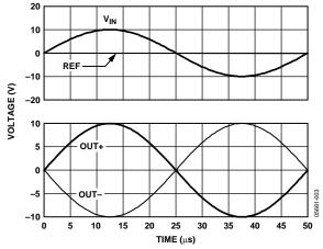
Figure 42. Typical Input/Output Response—Centered Reference
