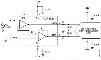
Figure 50. Driving a Differential Input ADC
