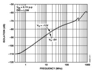
Figure 13. Isolation vs. Frequency—Disabled
