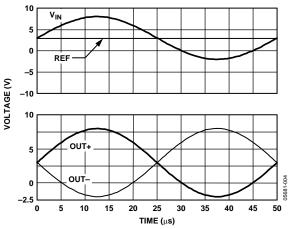
Figure 43. Typical Input/Output Response—Equal Input/Reference
