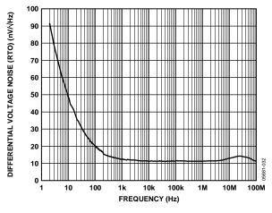
Figure 22. Differential Output Noise vs. Frequency
