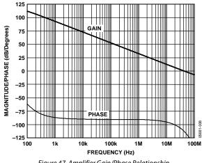
Figure 47. Amplifier Gain/Phase Relationship
