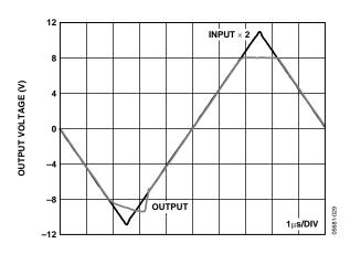
Figure 29. Input Overdrive Recovery,  $V_s = \pm 5 V$
