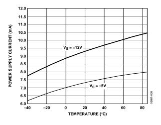
Figure 34. Power Supply Current vs. Temperature
