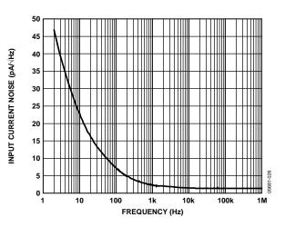
Figure 25. Input Current Noise vs. Frequency
