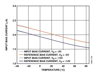
Figure 35. Input Bias Current vs. Temperature
