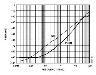
Figure 19. PSRR vs. Frequency
