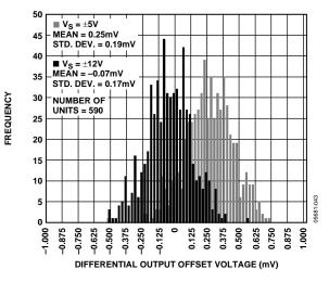
Figure 33. Differential Output Offset Voltage Distribution
