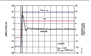
Figure 31. Settling Time,  $V_{\rm S} = \pm 12 V$
