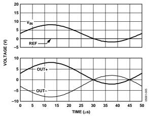
Figure 44. Typical Input/Output Response—Unequal Input/Reference
