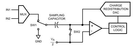
Figure 45. ADC122S021 in Track Mode
