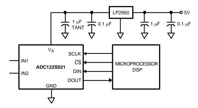
Figure 48. Typical Application Circuit
