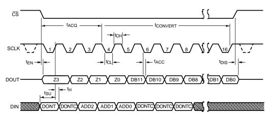
Figure 3. ADC122S021 Serial Timing Diagram
