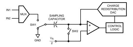
Figure 46. ADC122S021 in Hold Mode
