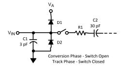
Figure 49. Equivalent Input Circuit
