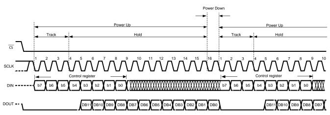
Figure 1. ADC122S021 Operational Timing Diagram
