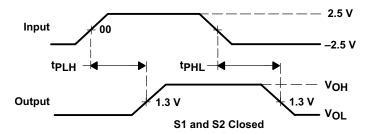
Figure 12. Voltage Waveforms For  $t_{\text{PLH}},\,t_{\text{PHL}}$
