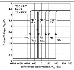
Figure 8. AM26LS32A Output Voltage vs Differential Input Voltage
