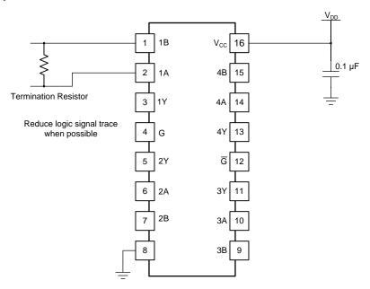
Figure 19. Layout with PCB Recommendations
