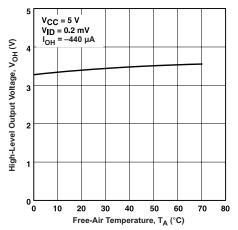
Figure 18. High-Level Output Voltage vs Free-Air Temperature
