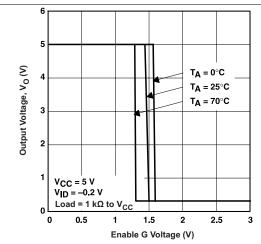
Figure 7. Output Voltage vs Enable G Voltage
