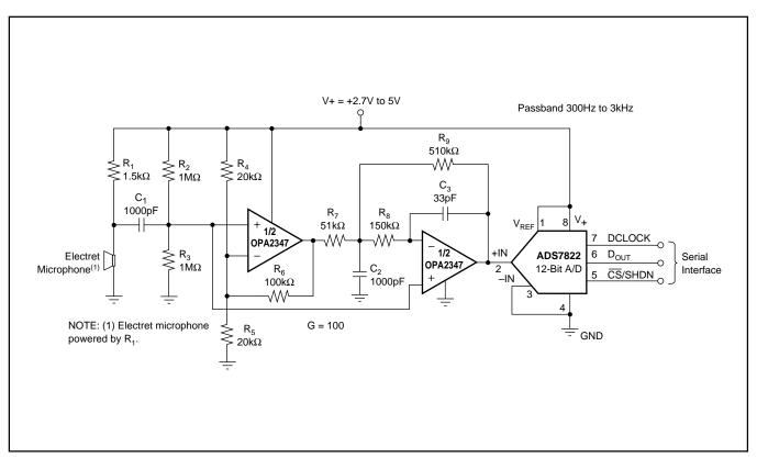
FIGURE 9. Speech Bandpass Filtered Data Acquisition System.
