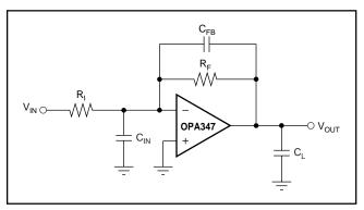
FIGURE 7. Adding a Feedback Capacitor In the Unity-Gain Inverter Configuration Improves Capacitative Load.
