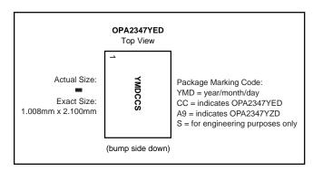
FIGURE 11. Top View Package Marking.
