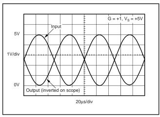
FIGURE 1. Rail-to-Rail Input and Output.
