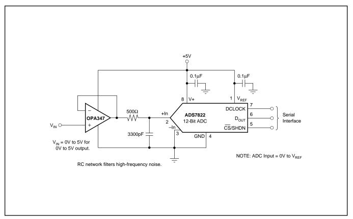
FIGURE 8. OPA347 in Noninverting Configuration Driving ADS7822.
