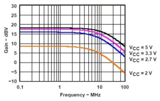
Figure 6. Open-Loop Gain
