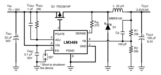
Figure 30. Typical Application Schematic for VOUT = 3.3V/500mA
