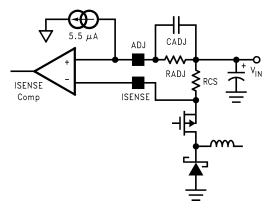
Figure 28. Current Sensing by External Resistor
