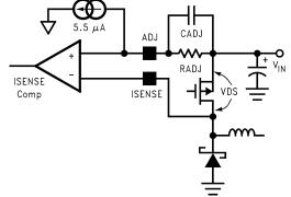
Figure 26. Current Sensing by V<sub>DS</sub>
