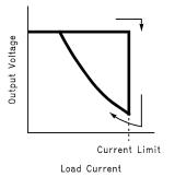
Figure 27. Current Limit Fold Back Phenomenon
