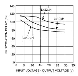
Figure 25. Propagation Delay
