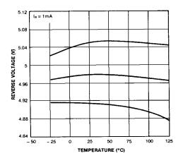
Figure 2. Temperature Drift
