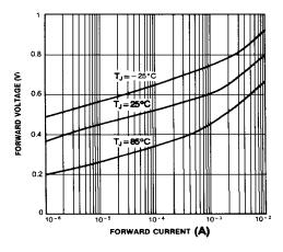
Figure 3. Forward Characteristics
