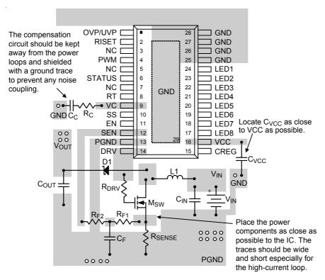
Figure 4. PCB Layout Guide
