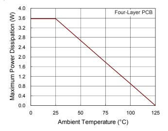
Figure 3. Derating Curve for RT8566 Packages
