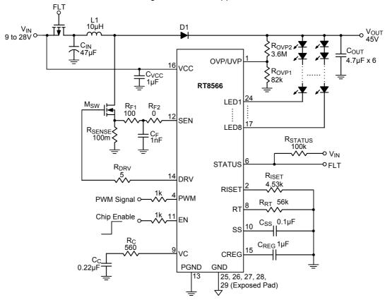
Figure 2. External P-MOSFET Isolation Application
