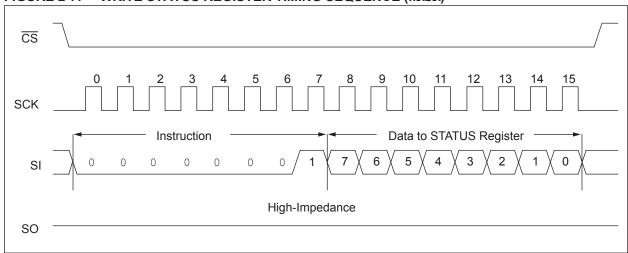
Note: An internal write cycle (Twc) is initiated on the rising edge of  $\overline{\text{CS}}$  after a valid write STATUS register sequence.
