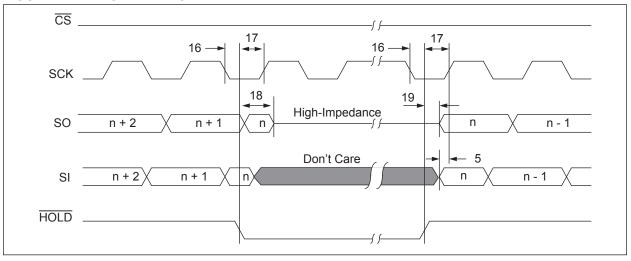
FIGURE 1-2: SERIAL INPUT TIMING
