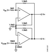
Figure 42. Single-Ended-to-Differential Configuration with the AD845
