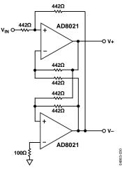
Figure 43. Single-Ended-to-Differential Configuration with the AD8021
