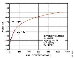
Figure 17. CMRR vs. Common-Mode Ripple Frequency
