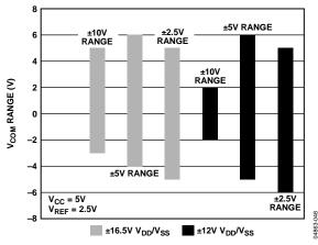
Figure 38. Common-Mode Range for  $V_{CC} = 5 \text{ V}$  and REFIN/OUT = 2.5 V
