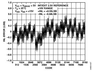
Figure 7. Typical INL True Differential Mode
