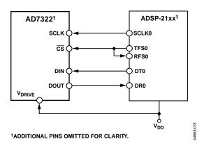
Figure 51. Interfacing the AD7322 to the ADSP-21xx
