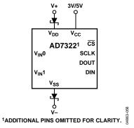
Figure 53. Schottky Diode Connection
