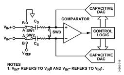
Figure 25. ADC Differential Configuration During Acquisition Phase
