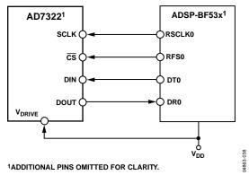
Figure 52. Interfacing the AD7322 to the ADSP-BF53x
