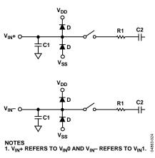
Figure 30. Equivalent Analog Input Circuit (Differential)
