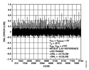
Figure 6. Typical DNL True Differential Mode
