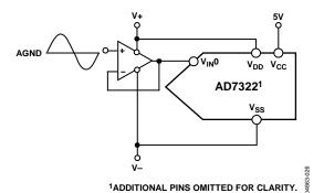
Figure 33. Single-Ended Mode Typical Connection Diagram
