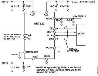
Figure 32. Typical Connection Diagram
