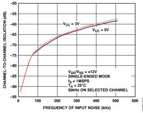
Figure 14. Channel-to-Channel Isolation
