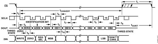
Figure 2. Serial Interface Timing Diagram
