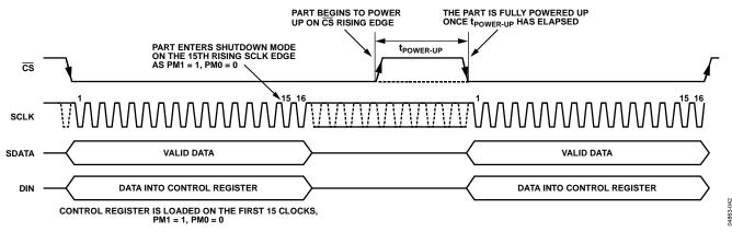
Figure 47. Entering Autoshutdown/Autostandby Mode
