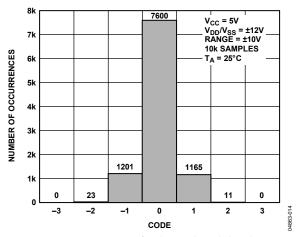
Figure 16. Histogram of Codes, Single-Ended Mode
