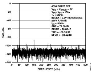
Figure 4. FFT True Differential Mode
