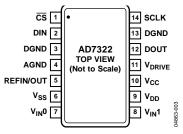
Figure 3. Pin Configuration
