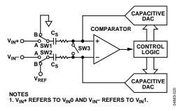
Figure 26. ADC Differential Configuration During Conversion Phase
