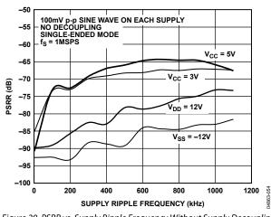
Figure 20. PSRR vs. Supply Ripple Frequency Without Supply Decoupling
