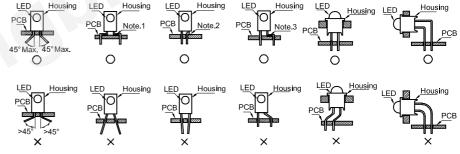
○ " Correct mounting method " x " Incorrect mounting method
