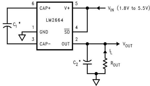
\*C<sub>1</sub> and C<sub>2</sub> are 3.3 μF, SC series OS-CON capacitors.
