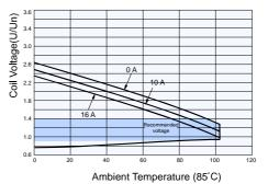
Notes: \* The use of a relay with an energising voltage other than the rated coil voltage may lead to reduced electrical life. An energising voltage over the abver range may damage the insulation of relay coil.
