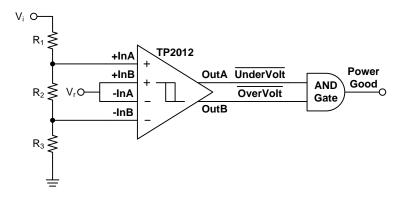
Figure 9. Windowed Comparator
