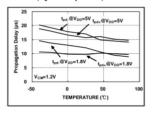
**Propagation Delay Skew vs. Temperature**
