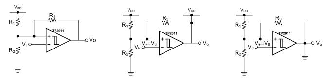
Figure 5. Inverting Configuration with Hysteresis
