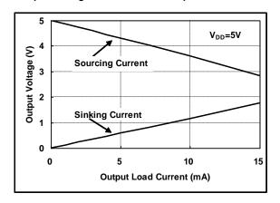
Output Voltage Headroom vs. Output Load Current
