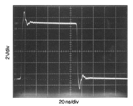
Figure 60. Improperly Terminated Signal
