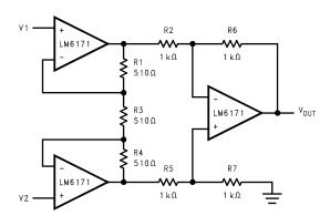
$$\begin{split} &V_{IN} = V2 - V1 \\ &\text{if R6} = R2, R7 = R5 \text{ and } R1 = R4 \\ &\frac{V_{OUT}}{V_{IN}} = \frac{R6}{R2} \left(1 + 2\frac{R1}{R3}\right) = 3 \end{split}$$
