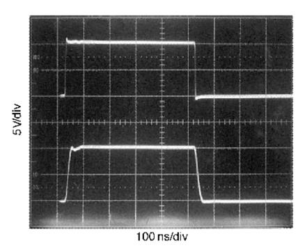
Figure 62. The LM6171 Driving a 200 pF Load with a  $50\Omega$  Isolation Resistor
