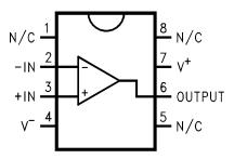
Figure 1. Top View 8-Pin SOIC/PDIP See Package Number D (SOIC) or See Package Number P (PDIP)
