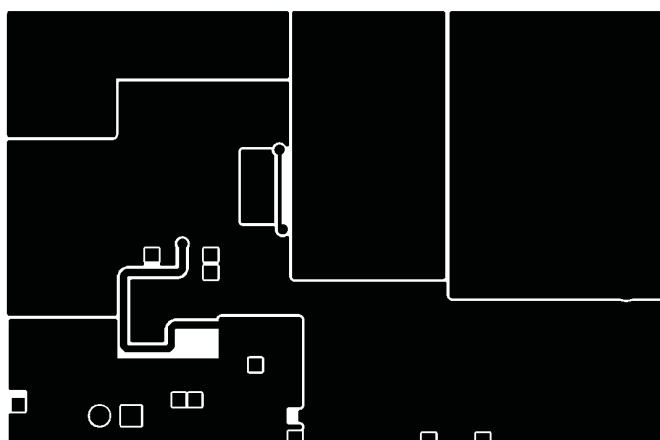
Figure 46. TPS40200EVM-001 Bottom Copper (X-Ray View from Top)
