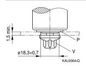
Insulated mounting with cap nut
