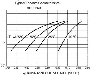
Figure 4 **Typical Forward Characteristics** MBR0530~MBR0540
