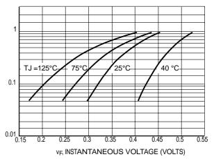
Figure 6 Typical Forward Characteristics
