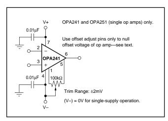
FIGURE 1. OPA241 and OPA251 Offset Voltage Trim Circuit.
