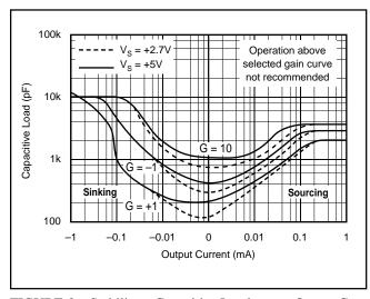
FIGURE 2. Stability—Capacitive Load versus Output Current for Low Supply Voltage.
