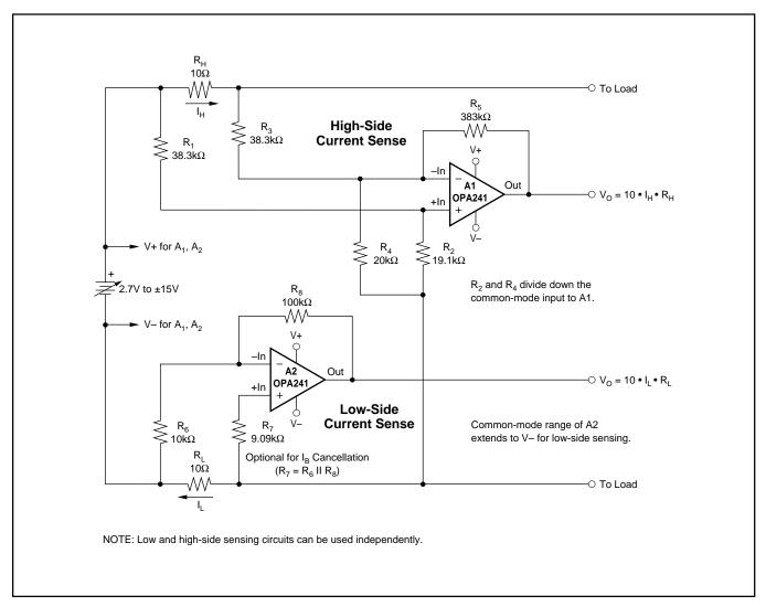
FIGURE 5. Low and High-Side Battery Current Sensing.
