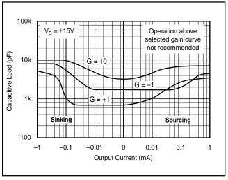
FIGURE 3. Stability—Capacitive Load versus Output Current for ±15V Supplies.
