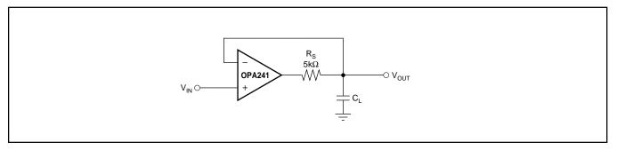
FIGURE 4. Series Resistor in Unity Gain Configuration Improves Capacitive Load Drive.
