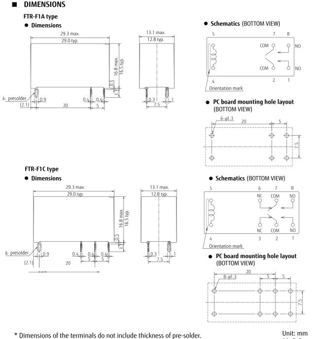
\* Tolerance of PC board mounting hole layout : ±0.1 unless otherwise specified.
