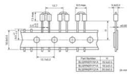
BL01/02/03 series are ferrite beads with lead wires to produce a high frequency loss for suppression of noise. Simple construction and easy-to-use, effective for low impedance circuits such as power supplies and grounds. Effective also for preventing overshoot and undershoot of digital signal in clocks or the like, and suppressing the higher harmonic wave. Suitable for prevention of abnormal oscillation at high frequency amplifying circuit.
